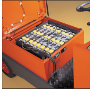
High battery capacity of 360 Ah. This means, depending upon the application conditions, running times of up to 8 hours. Multi-shift operation easily possible by simply exchanging battery tray.
