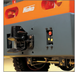
Heavy-duty Rockinger bolt coupling for towing loads up to 5 t. When attaching heavy transport vehicles, the reversing button proves to be especially handy. This makes it possible to guide the Hako Sherpa S5 on to the shaft from the rear.
