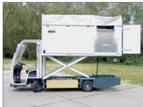
Hako-Cargo specialist vehicle with hydraulic lifting platform.
